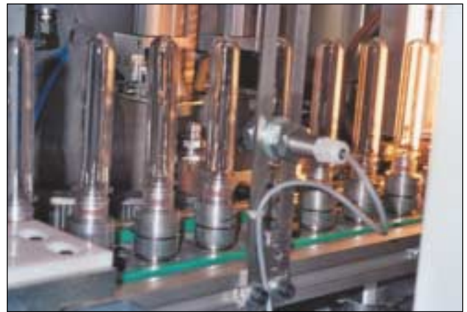
Left: Cad/cam solutions for 3D designing of the new Pakido range by Aisapack. Above: A user-friendly machine design featuring a single control point for all operations and accessibility to all components. Below left: Temperature control device ensuring that only the preforms with adequate temperature profiles are blown. Below right: Preforms being loaded onto the blowing fingers before entering the moulds.
