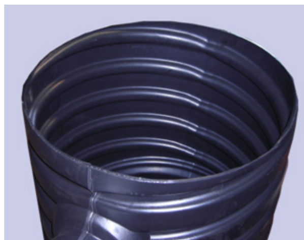
Part size variations meant that a fine focus laser could not be used when deflashing this drainage component.
